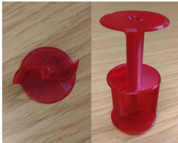
(b) Seed design printed by 3D printer; 35 mm in diameter; 70 mm tall; 7 g; 45-min printing time at 0.3-mm resolution.
