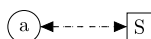
Figure 4. A combination of a read, a push, and a pull edge, abbreviated as a double-headed information edge.
