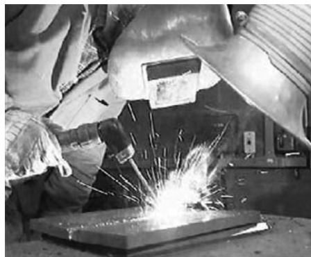
Fig. 1.6 Welding using shielded metal arc welding process
