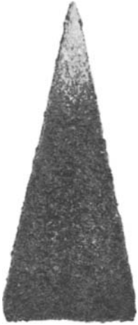
Figure 1-35 Fractograph of wedge test specimen of cast iron. The white areas indicate the presence of iron carbide, while the dark areas indicate that flake graphite is present.
