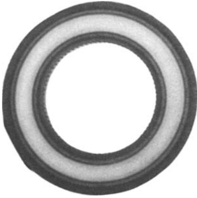
Figure 1-29 Macroetching (10% aqueous \text{HNO}_3 ) of a disc cut from this carburized AISI P2 part revealed a heavy case at both the ID and OD. The surface was 65.5 HRC (Rockwell hardness on the C scale) while the center was at 85 to 86 HRB (Rockwell hardness on the B scale).
