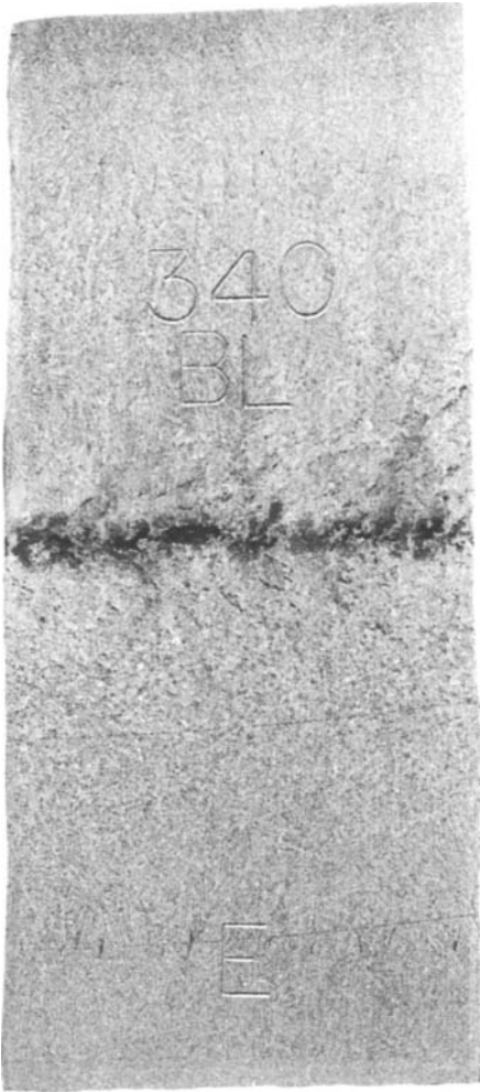
Figure 1-12b Hot-acid etching of a longitudinal disc from the center of the disc shown in Fig. 1-12a revealed the extent of the open center condition. (Courtesy of M. Schmidt, Bethlehem Steel Corp.)
