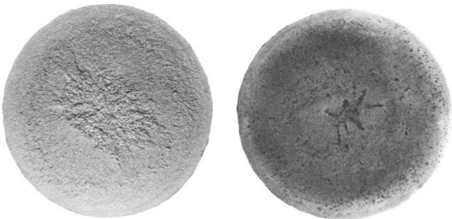
Figure 1-37 The fracture of this eutectoid carbon bar that broke during heat treatment reveals the depth of hardening and an unsound center condition. Hot-acid etching of a disc from behind the fracture reveals the unsound center and extensive segregation.
