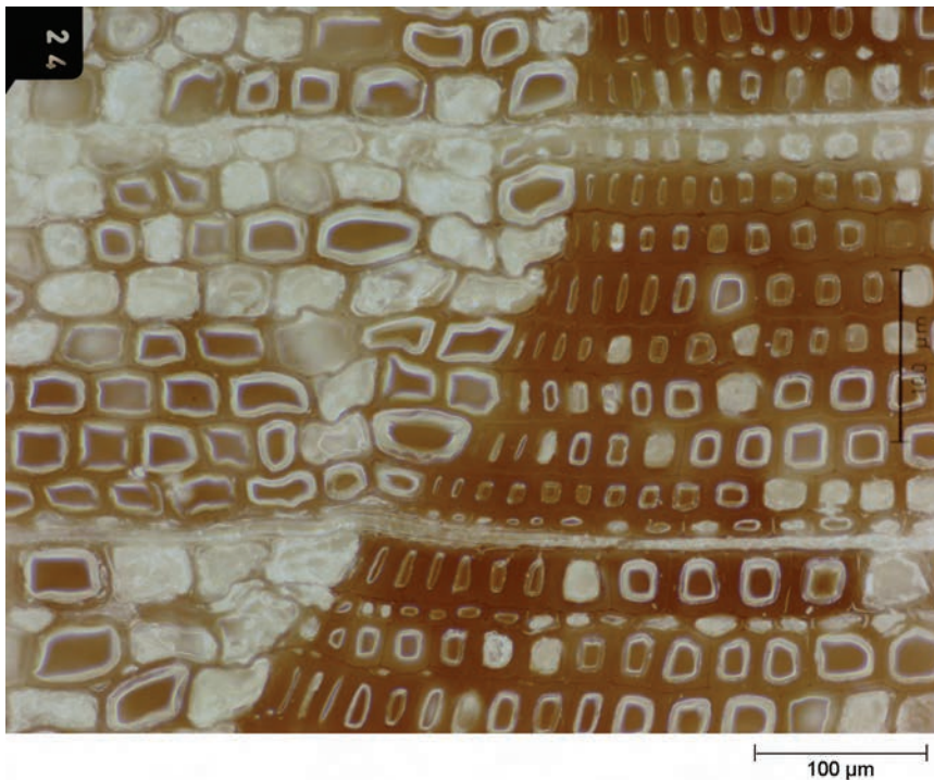
Fig. 1.16 Ultrathin section showing the microstructure of spruce wood. Transmitted-light phase contrast, 40× objective
