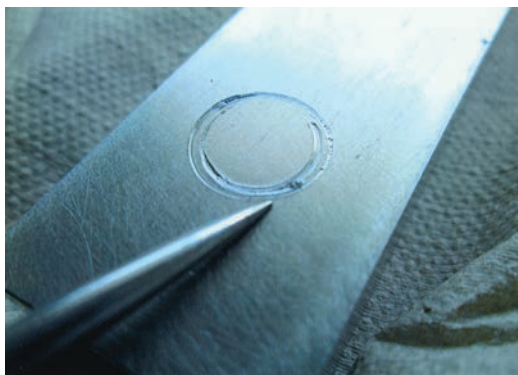
Fig. 1.4 Galling formation of excrescences from rubbing contact with another metal
