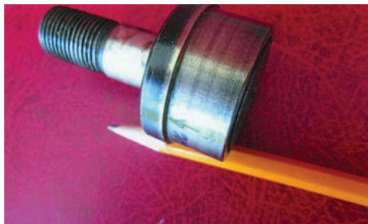
Fig. 1.8 Wear of a cam follower. There was no step in the outside diameter when it was new.
