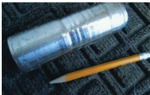
Fig. 1.2 Abrasion of a stainless steel pump sleeve by glass-filled packing
