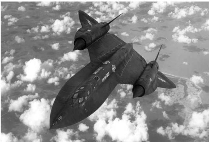
Fig. 1.1 SR71 aircraft: first use of beta alloys in aerospace structures. Courtesy of Lockheed California Co.
