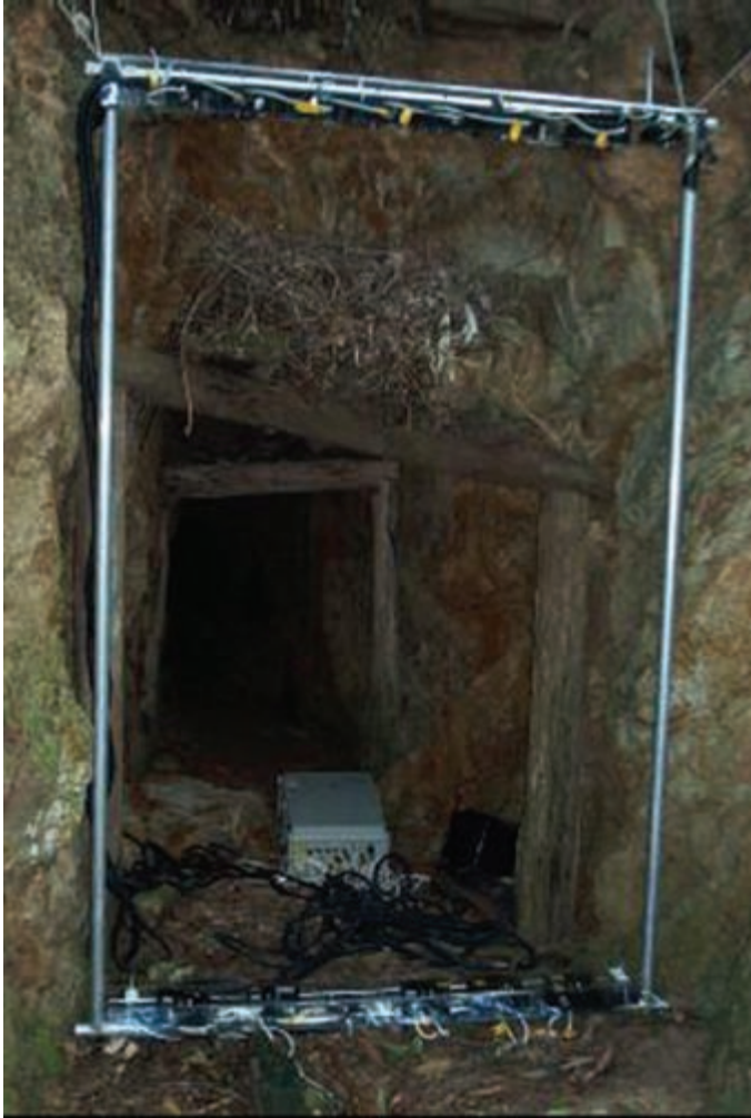
Infrared Counter and data logger at Mumbulla Mine. Note Superb Lyrebird nest above entrance.
