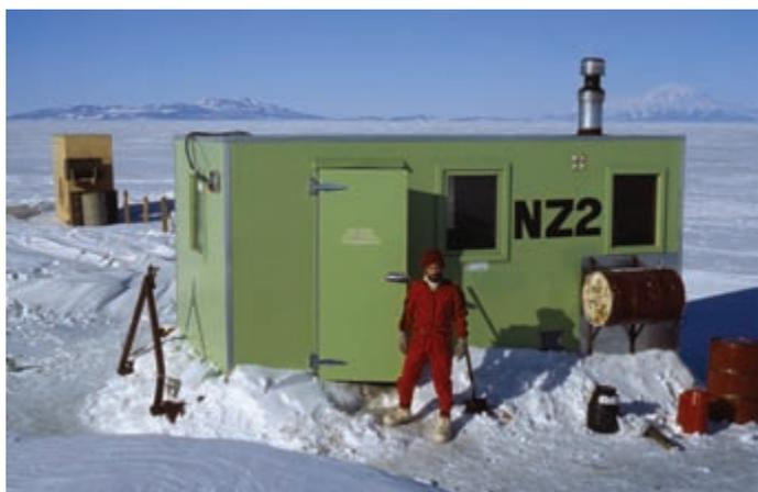
**Figure 4.** A portable laboratory with a 7.5 kVA diesel power generator was set up over a fishing hole drilled through the 2 m thick ice cover on the Ross Sea, Antarctica. The hut was heated to prevent the seawater from re-freezing and to allow the researchers to conduct physiological experiments.
