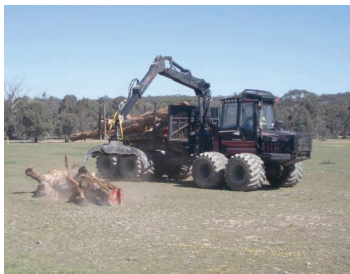
Figure 4 – Placement of logs on an experimental site with forestry forwarder. Photo, A. Manning.
