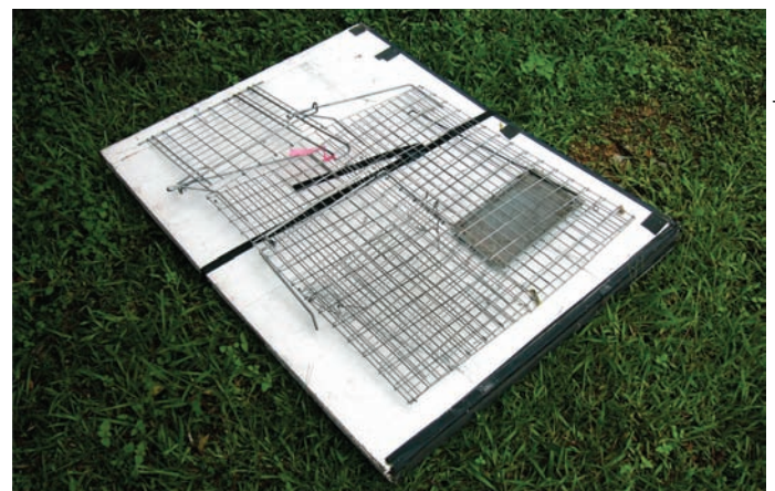
Figure 1. Koala trap dismantled and ready for storage and/or transport; the total weight of all components is approximately 15kgs.
