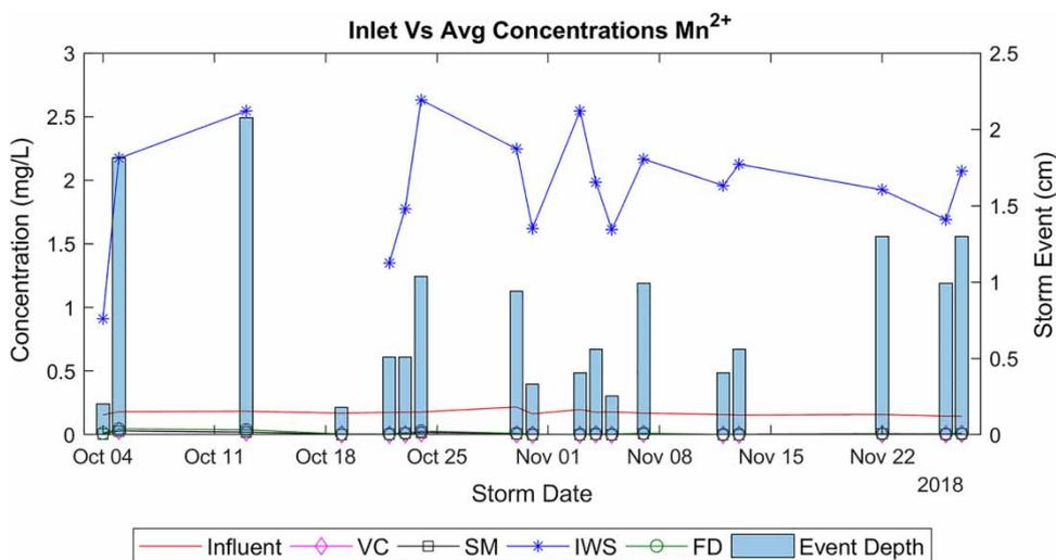
**Figure 7** |  $\text{Mn}^{2+}$  outlet concentrations for all treatment types.
