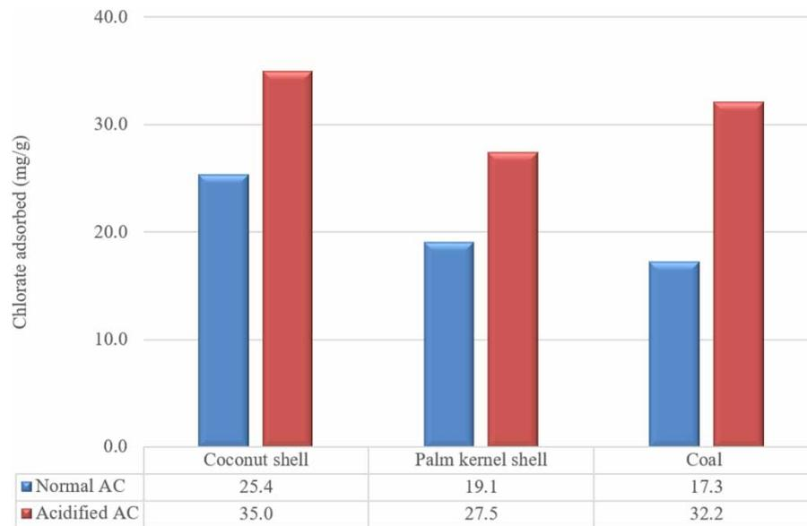
**Figure 4** | Comparison of chlorate adsorbed between normal and acidified activated carbon.
