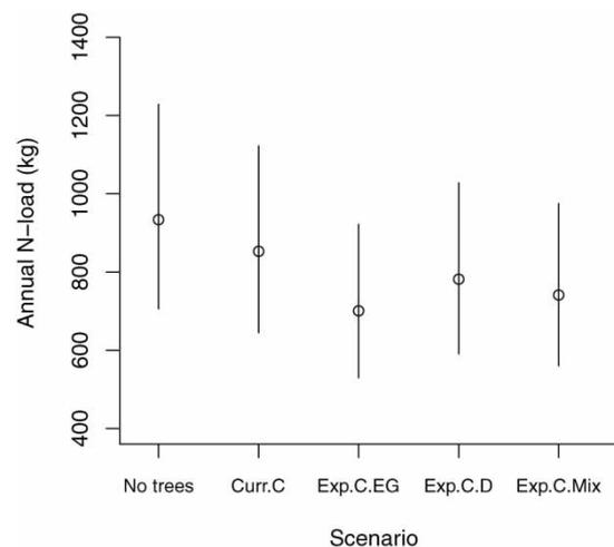
**Figure 6** | Predicted range of annual N-load from the impervious parts of public land within the Elizabeth Street Catchment. Trees covering hard surfaces provide some N-load avoidance through interception (Curr.C), with further reductions possible with canopy expansion using only evergreens (Exp. C. EG), only deciduous (Exp. C. D) or equal mix of deciduous and evergreen trees (Exp/ C. Mix).
