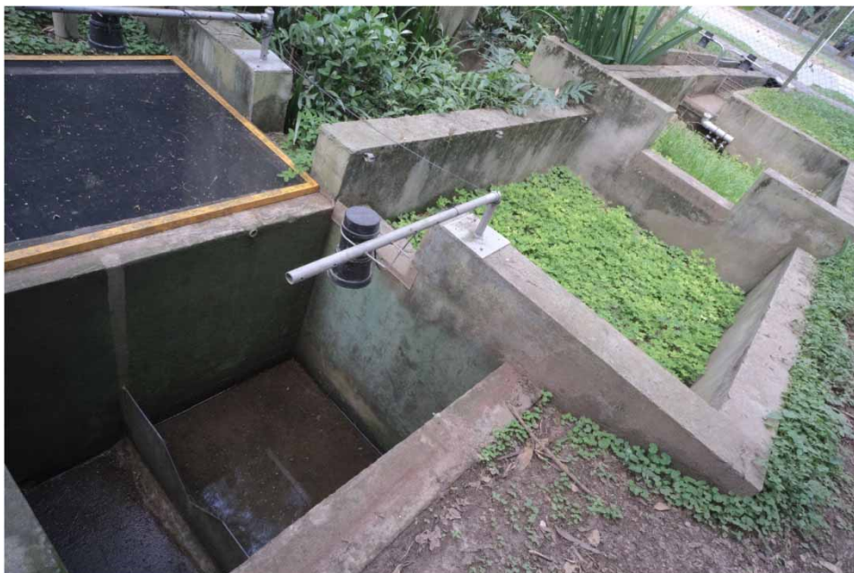
Figure 9 | Bioretention using the same method for water quantity characterisation: the inlet with a rectangular-notch acrylic thin-plate weir surrounded by a concrete framing and the outlet with a triangular-notch steel thin-plate weir in a concrete tank. Source: the authors.
