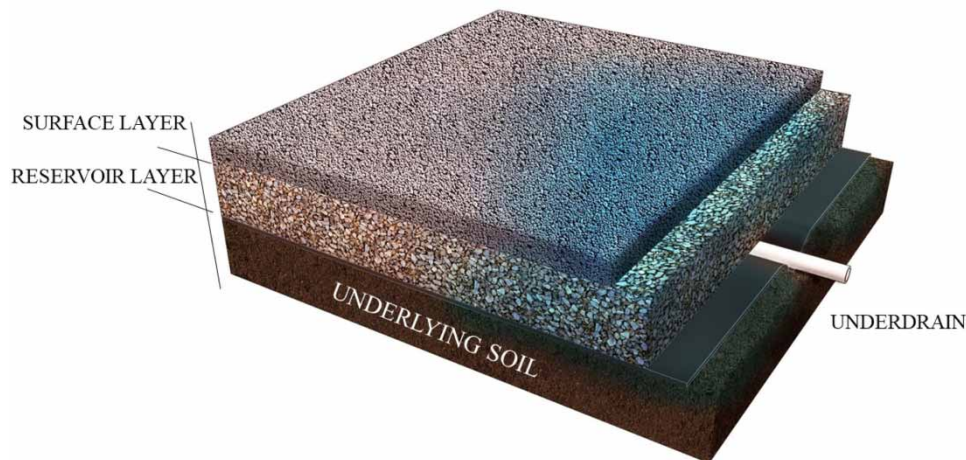
Figure 1 | Permeable pavement system typical cross-section with a permeable concrete surface, permeable reservoir with open-graded coarse aggregates, and underdrains.
