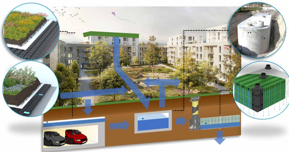
Figure 3 | Blue-green infrastructures considered: extensive green roof; green roof on top of an underground parking; infiltration trench and a storage infrastructure. The graphic shows the water flow in a model urban residential block (images of the technologies were provided by www.optigruen.de and the image of the residential block provided by 'silisight for msm Architekten' and modified accordingly by Breulmann M & Khurelbaatar G). S_{tot} : total storage; S_{ret} : retention storage; S_{sub} : substrate storage; kc_{vegetation} : vegetation coefficient; SR: storage coefficient of the filling material and K_f : permeability coefficient.
