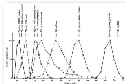
Gel filtration: elution of neutral molecules in order of descending molecular masses, from columns of untreated potato starch in water. From Lathe and Ruthven<sup>4</sup>, Figure 1 © 1956 The Biochemical Society
