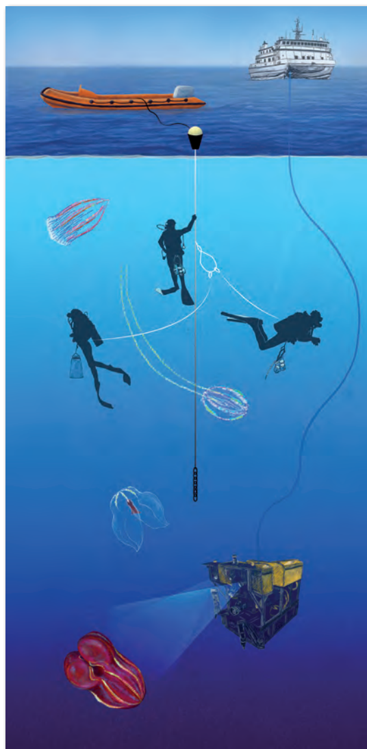
Figure 1: Ctenophore collection using the remotely operated vehicle (ROV) Doc Ricketts and blue-water diving techniques. Scuba divers can collect between the surface and 20 metres depth, while Doc Ricketts captures specimens and video down to 4000 metres. Ctenophore size is exaggerated in this schematic. Illustration by Kelly Lance, MBARI.
