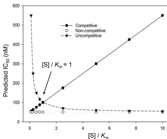
**Figure 1.** Predicted  $IC_{50}$  values for various inhibitor types at various substrate concentrations, assuming  $K_i = 50$  nM. The predicted  $IC_{50}$  value for mixed inhibitors depends on the proportion of competitive and non-competitive components of inhibition.
