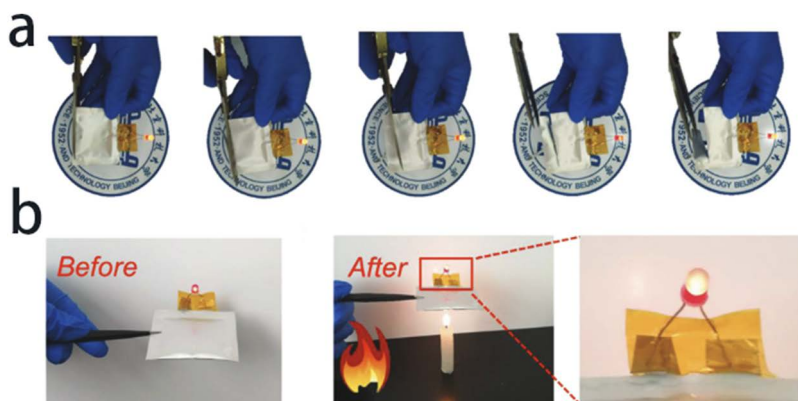
Figure 4.22 (a) Cutting off part of a solid-state aluminium-ion battery can steadily power a light-emitting diode (LED) lamp. (b) Solid-state aluminium-ion batteries for lighting LED lights when burning in a fire. Reproduced from ref. 135 with permission from John Wiley & Sons, Copyright 2019.
