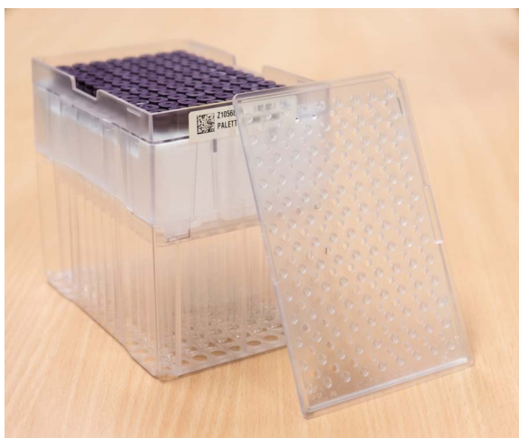
Figure 1.1 96 tube sample rack containing 5 mm sample tubes developed to enable sophisticated automation of the NMR preparation and acquisition process of biofluids.
