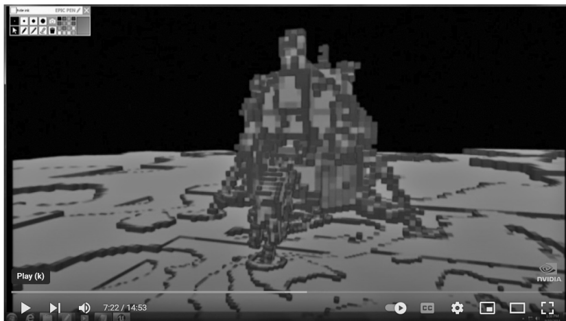
4.2 Screenshot of the moon landing demo’s “voxel” mode, which shows the different boxes of light that serve as base calculation units for rendering the scene. ( https://www.youtube.com/watch?v=QIap1jL14WU )
