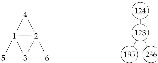
**Figure 5** Left: A graph  $G$  for which no inside tree decomposition is optimal. Right: An optimal tree decomposition for  $G$ . Note that, regardless of which bag is chosen as the root, there exists a vertex  $v$  such that the bags containing  $v$  are not all on a path from the root to a leaf.
