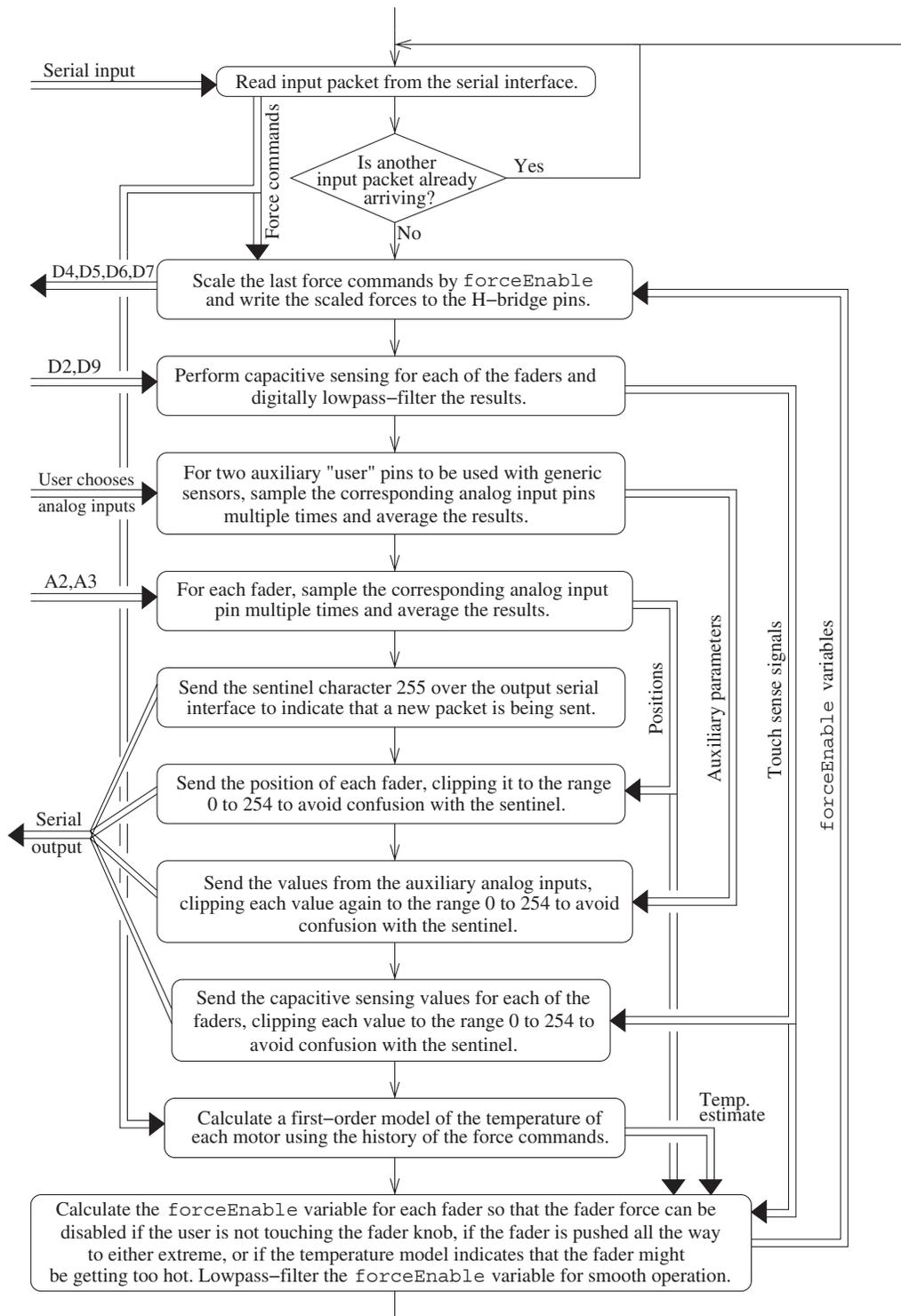
if the software got stuck trying to push the fader knob beyond the end of travel. Finally, a simple temperature model uses the history of the force commands to produce an approximate temperature estimate (see Figure 7), which is used to turn off the force if the fader motor might be getting too hot because of a prolonged period of large force exertion.
