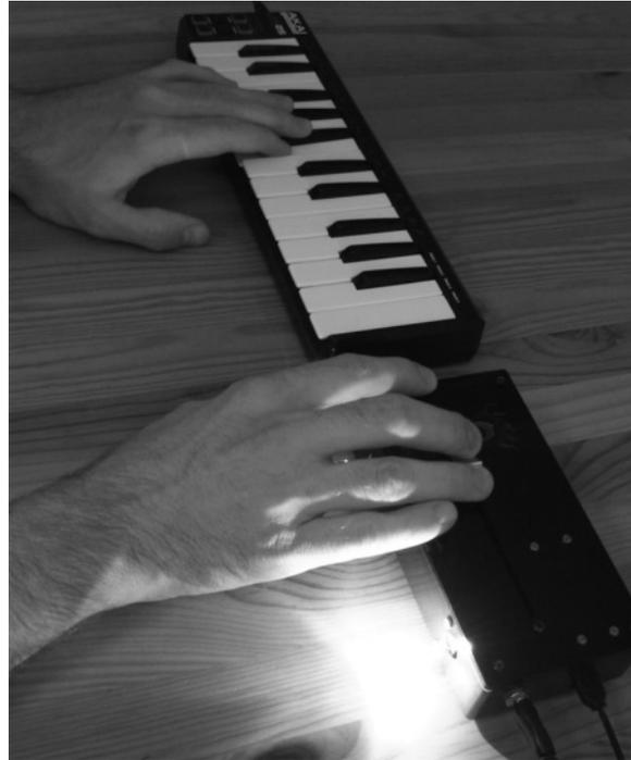
presents an example configuration combining a FireFader prototype with a small MIDI keyboard.
