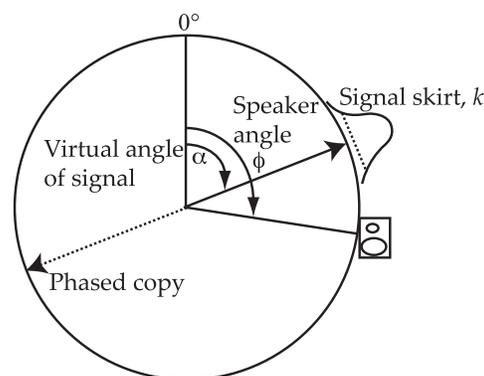
first calculates whether the speaker is within the skirt of the virtual angle. It then uses a cosine curve to calculate the amplitude of the texture stream for that speaker. I named this abstraction `weightor~`. The simple calculation is
