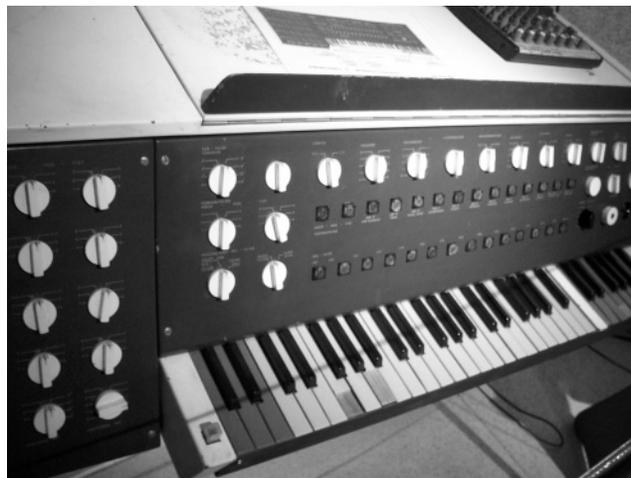
to develop a new musical instrument called the Subharchord, which generated sounds electronically (see Figure 2). This instrument was actually built, and it formed the center of a working studio. That was a laboratory for research and development.
