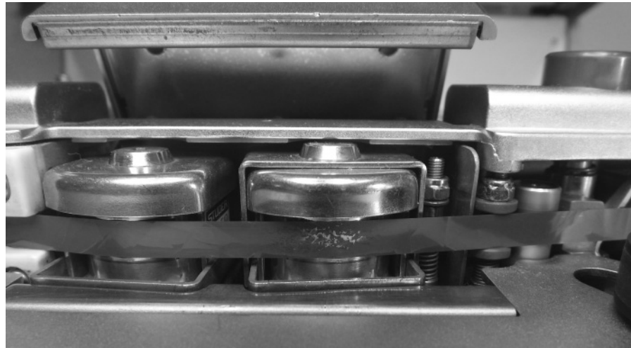
Figure 1. Creases on a tape and localized magnetic coating damage. (Color version available at www.mitpressjournals.org/doi/suppl/COMJ_a_00487-Preitto .)
