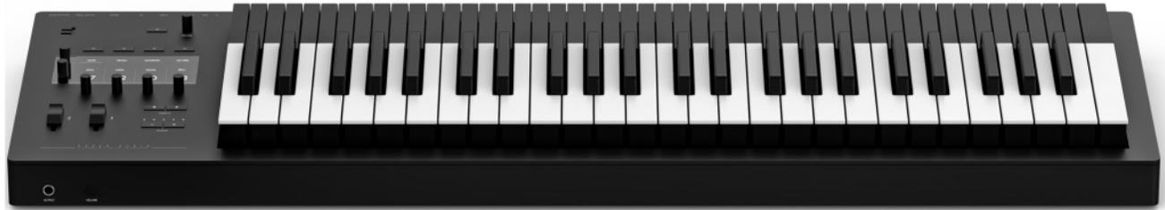
The keyboard has a built-in color LCD screen, eight encoders, and nine buttons for controlling settings. The user can configure MIDI equipment directly, without the need for a computer. Osmose supports multichannel MPE and MPE+, and it can send polyphonic aftertouch and global pitch bend messages. Alternatively, the keyboard can be used in piano mode, in which it acts like a simple keyboard controller, sending velocity messages for each note.
