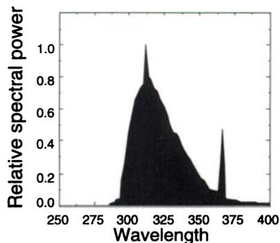
Fig. 1. Emission spectrum of the Westinghouse FS20 UVB source after transmission through a bacteriological grade Petri dish.
