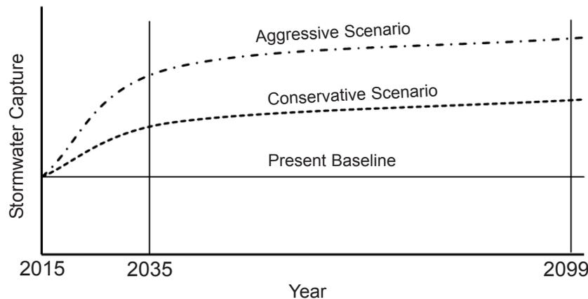
The Stormwater Capture Master Plan (SCMP) considers scenarios that, using aggressive action, could nearly triple the amount of stormwater captured. Source: Rafael Villegas, *Stormwater Capture Master Plan: The Master Planning Process* (Los Angeles: Los Angeles Department of Water and Power, 2014).
