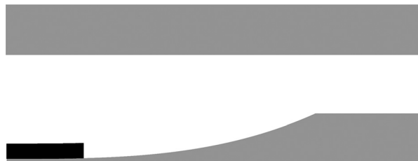
Fig. 1. Unmodified beam profile (top) and optimal thickness profile (bottom). The left-hand side is modelled as free and the right-hand side is modelled as clamped in the calculation of W . Dimensions are not to scale.
