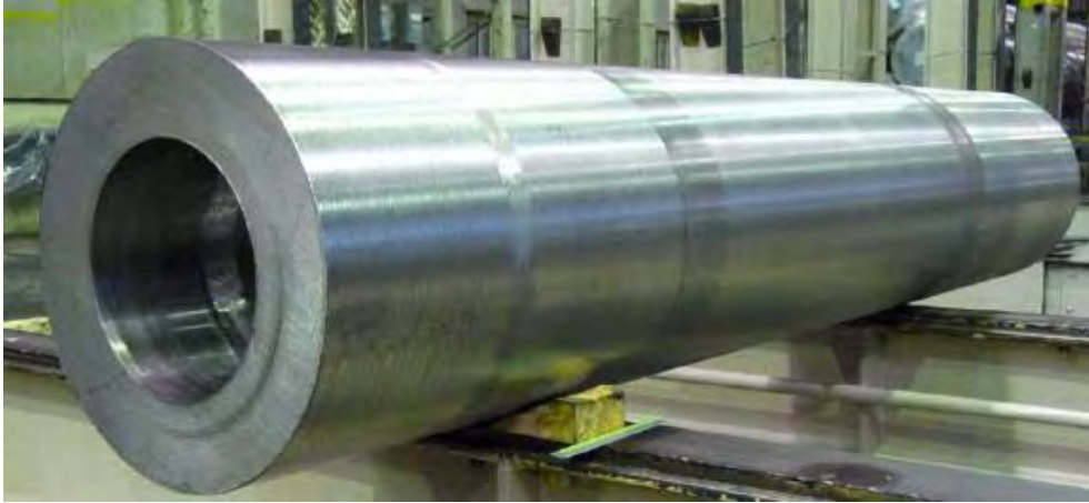
Figure 8: HR6W pipe – experimental component (courtesy of NSSM co.) [2]
