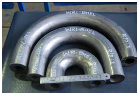
Figure 2: Alloy 617M Tubes Cold Bent to R/D 1, 2 and 3
