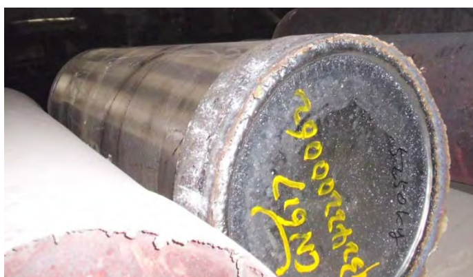
Figure 9 CN617 alloy ingot after VIM+VAR (Courtesy of CISRI and Fushun Special Steel, 2013)
