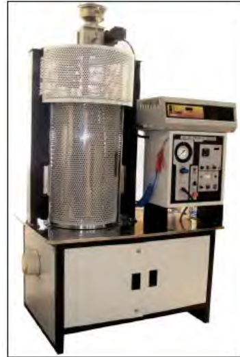
Figure 12. Test system used at DUCOM, (200 m/s; 800C max.)
