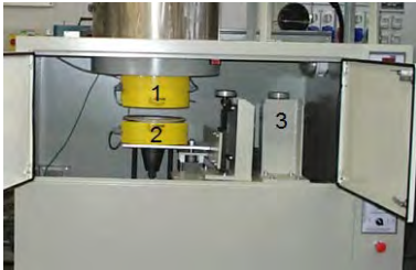
Figure 11. Test system at ERSE SpA, Mila, Italy, (200 m/s; 800C max.)
