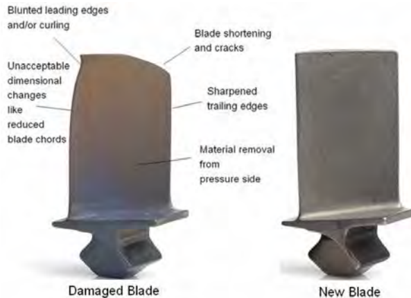
Figure 3 Comparison of compressor blade damaged by SPE (left) with a virgin blade (right) [10]
