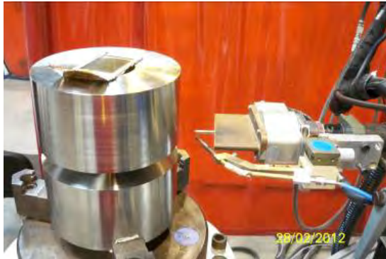
Figure 2: Configuration of welding samples Nimonic 263 + Nimonic 263 Ø160mm on experimental welding stand with narrow gap torch.
