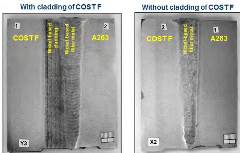
Figure 8: Macrostructure of dissimilar weld joint A263 + COST F taken for both variants with/without cladding of COST F.
