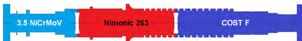
Figure 1: Dissimilar weld joint Nimonic 263 + COST F applicable for IP turbine of A-USC power plant.
