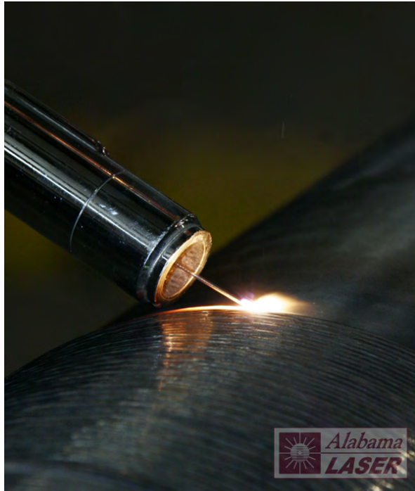
Fig 9. Hot Wire Laser Beam Weld Overlay using INCONEL Filler Metal 72M.
