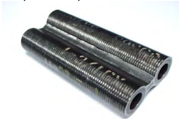
Figure 3. Water-wall panel section overlaid using INCONEL Filler Metal 72M via the automatic GTAW process. The membrane weld was performed using the SAW process.
