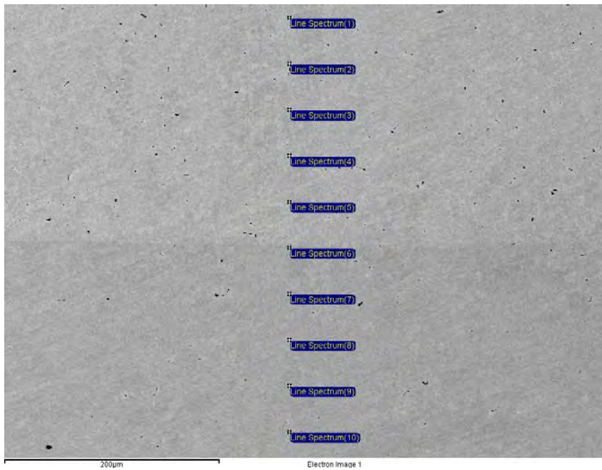
Fig 10. Longitudinal Cross-Section of 72M Overlay.
