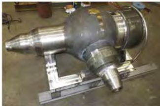
Fig. 21 Turbine bypass valve (Courtesy of ABB Bailey Japan)
