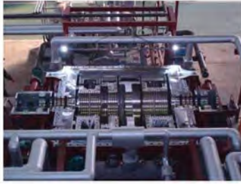
Fig. 25 Turbine rotor test facility under construction [4]
