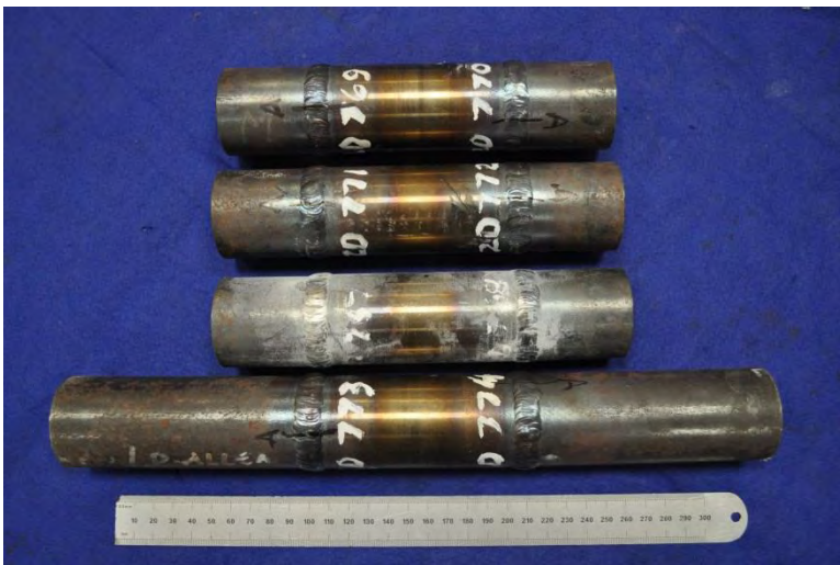
Figure 5: MarBN tubes from forged bar [6]
