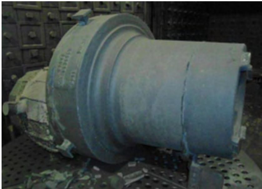
Figure 2: MarBN 8 tonne bonnet casting
