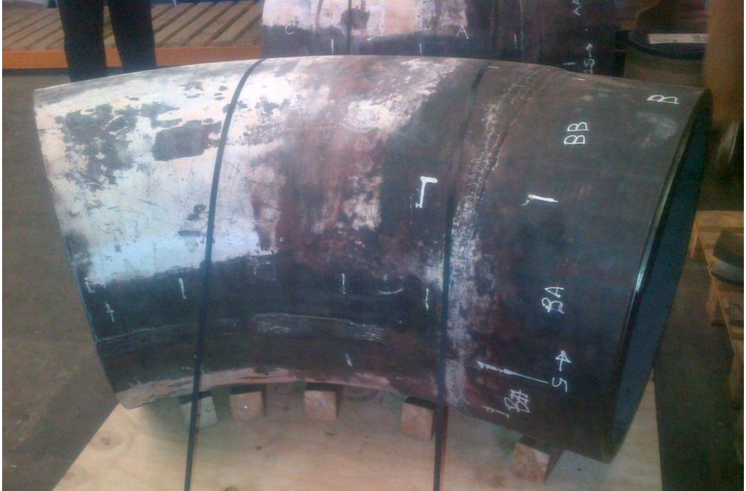
Fig.1. The bend, cut into two halves for ease of handling. The seam weld at the bend intrados and one of the circumferential welds can be seen.
