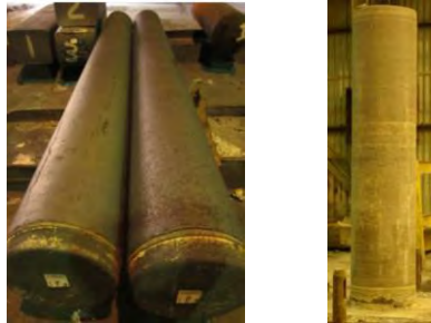
Figure 1: Two VIM electrodes (left) were remelted into two ESR ingots (right).
