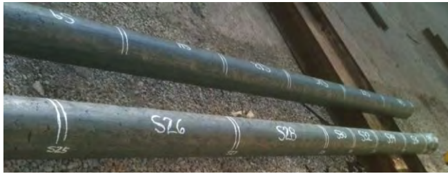
Figure 3: Triple melted ingots forged to 203 mm diameter for macro-segregation evaluation.
