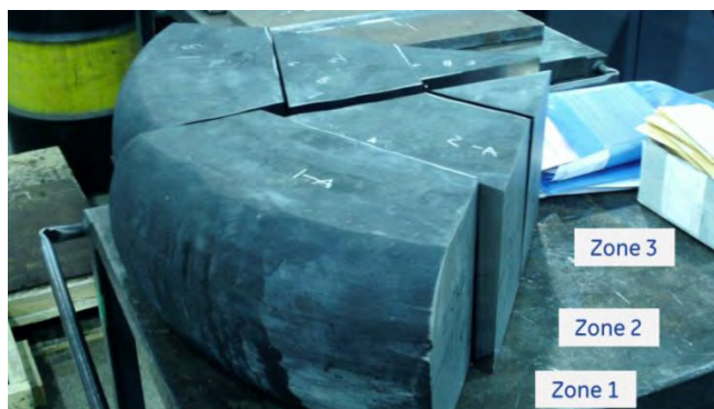
Figure 8: Final forged disk, shown cut into various zones for property evaluation.
