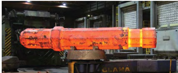
Figure 9: HP-rotor at final forging, COST steel E.
