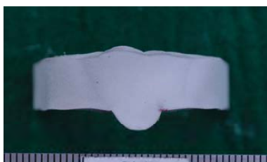
Figure 9 Appearance of SAVE12AD similar welded joint after bending test
