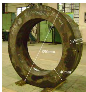
Figure 1: Dissimilar welded rotor of FB2 and 2.25Cr2NiMo1V steel.
