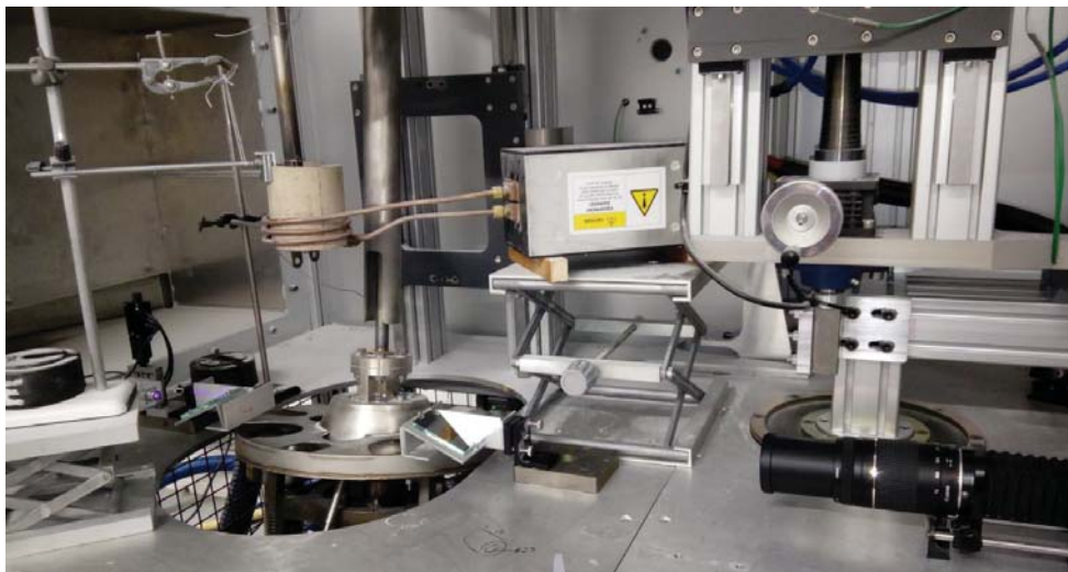
Figure 8 Internal view of the HTSPE apparatus showing the induction heater, sample hang down and laser optics.
