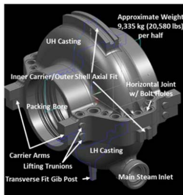
Figure 6: Trial Casting will be Lower Half of Nozzle Carrier (courtesy of GE)
