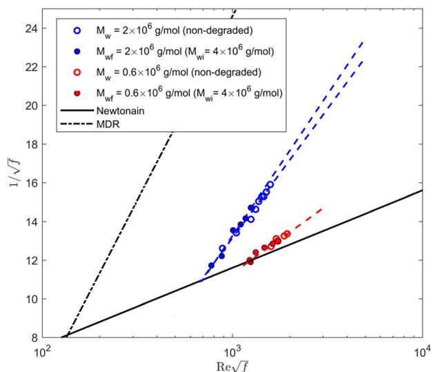
**Fig. 8 P–K plot comparing a steady-state degraded sample from a  $C = 100$  ppm PEO polymer ocean in a recirculating water tunnel with that of a nondegraded sample**
