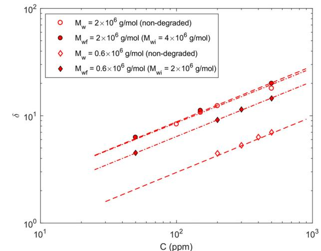
**Fig. 6 Slope increment versus concentration ( $C$ ) for degraded and nondegraded samples of  $M_w = 0.6 \times 10^6$  or  $2.0 \times 10^6$  g/mol. The dashed lines are all best fit curves with a slope of  $\sim 0.5$ .**
