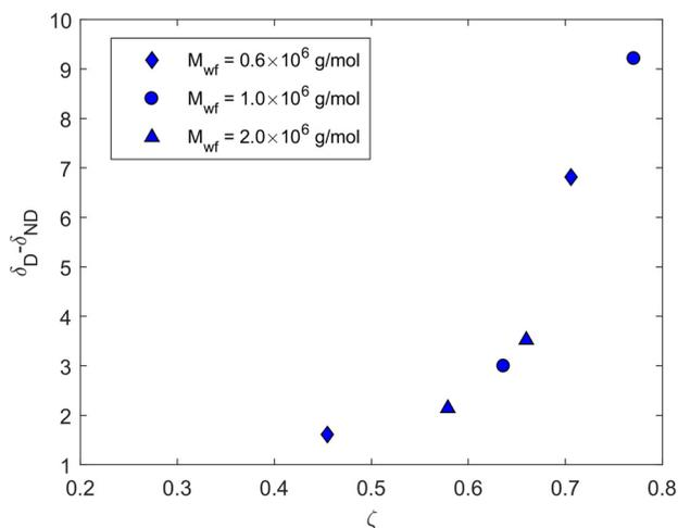
**Fig. 7** The difference between the degraded and nondegraded slope increments for  $C = 500$  ppm plotted versus the normalized difference between the initial and final molecular weights,  $\zeta = (M_{wi} - M_{wf})/M_{wi}$
