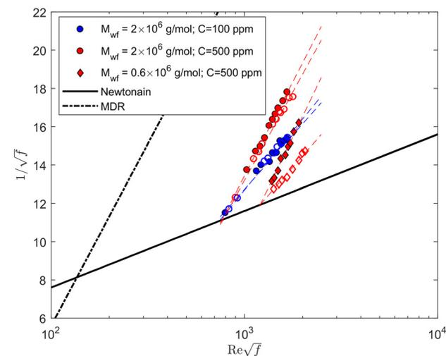
**Fig. 5 P–K plot comparing degraded and nondegraded samples with  $M_{wf} = 2 \times 10^6$  g/mol (degraded samples had  $M_{wi} = 4 \times 10^6$  g/mol) or  $0.6 \times 10^6$  g/mol (degraded sample had  $M_{wi} = 2 \times 10^6$  g/mol). Filled markers represent degraded samples.**
