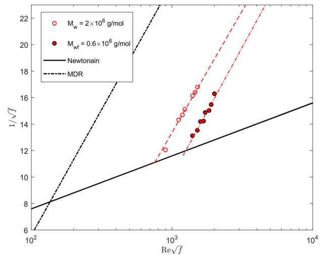
**Fig. 4 P–K plot using PEO at an initial  $M_{wi} = 2 \times 10^6$  g/mol and  $C = 500$  ppm. One of the samples was degraded to a lower molecular weight ( $M_w = 0.6 \times 10^6$  g/mol) while the other was nondegraded.**
