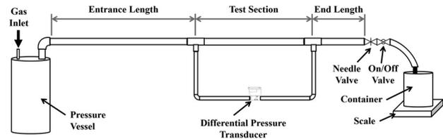
**Fig. 2 Schematic of the pressure drop apparatus used for characterization of the polymer samples as well as mechanically degrading samples**
