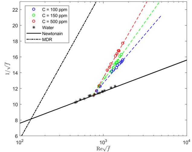
**Fig. 3** P–K plot of  $2 \times 10^6$  g/mol PEO at concentrations of 100, 150, and 500 ppm, as well as water (Newtonian) data at the same range of  $\text{Re}\sqrt{f}$ . Included for reference are the P–K law, MDR asymptote, and logarithmic best-fit curves to the data within the polymeric regime.
