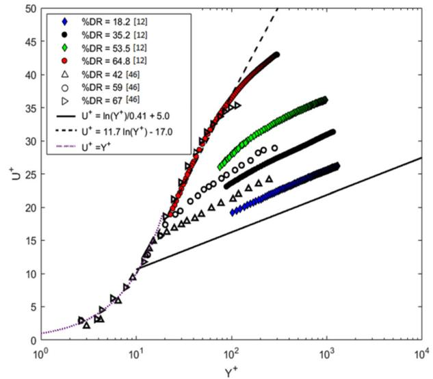
**Fig. 1 Polymeric velocity profiles from a turbulent boundary layer with nonuniform concentration distribution [12] and channel flow with a constant concentration [46], which shows an increasing slope with increasing drag reduction for HDR (DR > 40%)**
