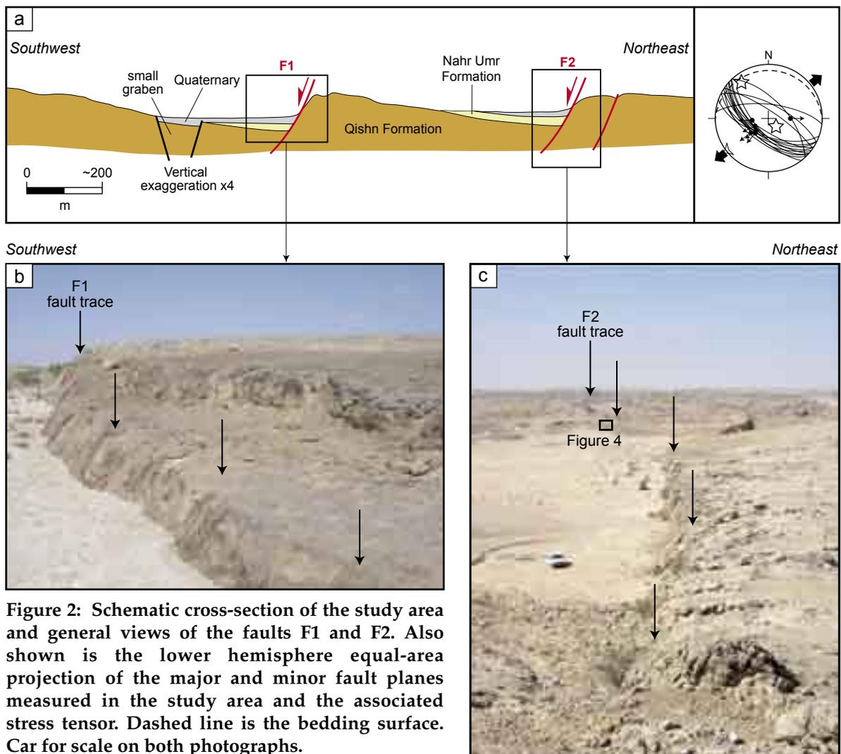
Figure 2: Schematic cross-section of the study area and general views of the faults F1 and F2. Also shown is the lower hemisphere equal-area projection of the major and minor fault planes measured in the study area and the associated stress tensor. Dashed line is the bedding surface. Car for scale on both photographs.
